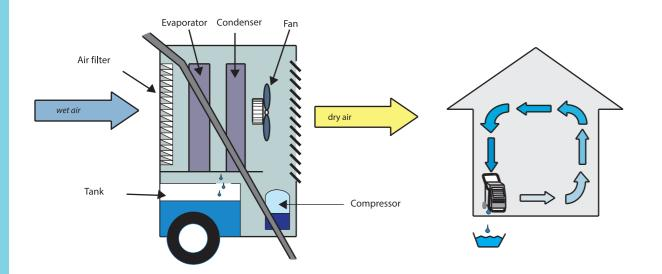
Wet air can cause damage of buildings and products and decrease the efficiency of production processes. LEWACO dehumidifiers are the best solution to fight the harmful moisture effects.
